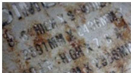
Road Salt Corrosion Damage
